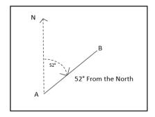
Let's review what a bearing is. In mathematics, a bearing is the angle in degrees measured clockwise from the north. Bearings are usually given as a three-figure bearing. For example, 30° clockwise from the north is usually written as 030°. Bearings are commonly used when traveling by plane, boat, or just navigating a hike.
