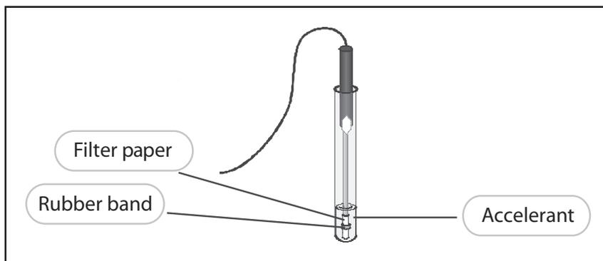
5. Pour a small amount of the accelerant from Suspect 1 into a test tube. Place the test tube in a test-tube rack, and place the temperature probe into the test tube so that the filter paper is covered by the liquid.
